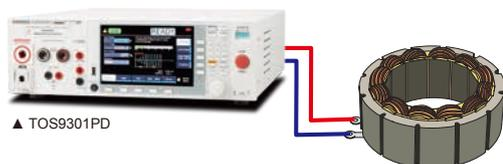
[Partial discharge voltage-Conceptual diagram of current characteristics]
