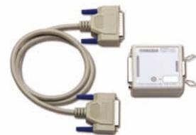
This is a terminal unit for converting a 25-pin SIGNAL I/O connector of TOS5300/5301/5302/5200 to a 14-pin SIGNAL I/O connector of TOS5050A/5051A. By connecting via this product, the external control performed with TOS5050A/5051A can be performed with TOS5300/5301/5302/5200 at the same time.
